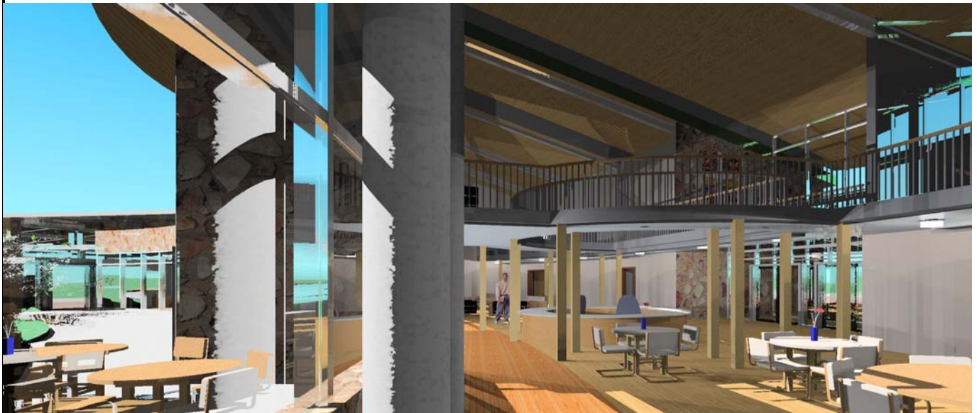
View of Dining room and main public zone, showing FSC certified wood and/or bamboo flooring, lodge-like interior design, and a southern window wall with shading louvers.
